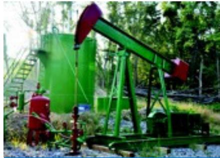
Pumpjacks like this can be found in many parts of western Pennsylvania, extracting oil from shallow geological formations. Some shallow wells produce both oil and natural gas; these wells often remain in production for decades.
